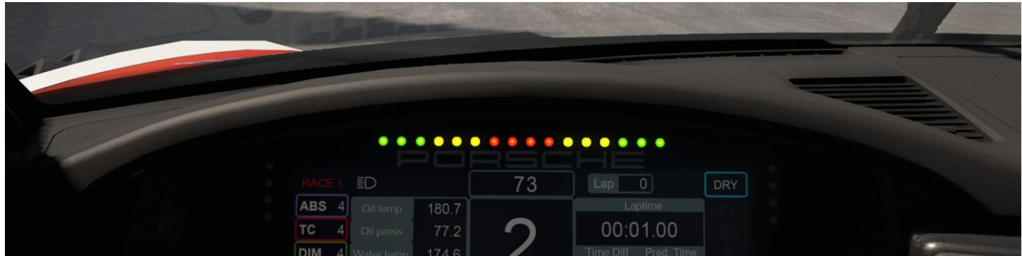
A row of multi-colored LEDs provide a visual representation of the engine's RPM and indicate when the engine has reached the optimum point for shifting. When all the LEDs at the top of the dash display flash blue, shift up. This is at 7900 rpm for 1st gear, 8200 rpm for 2nd gear, 8400 rpm for 3rd gear, 8500 rpm for 4th gear and 8600 rpm for 5th gear. 6th gear has specific behaviour to indicate
