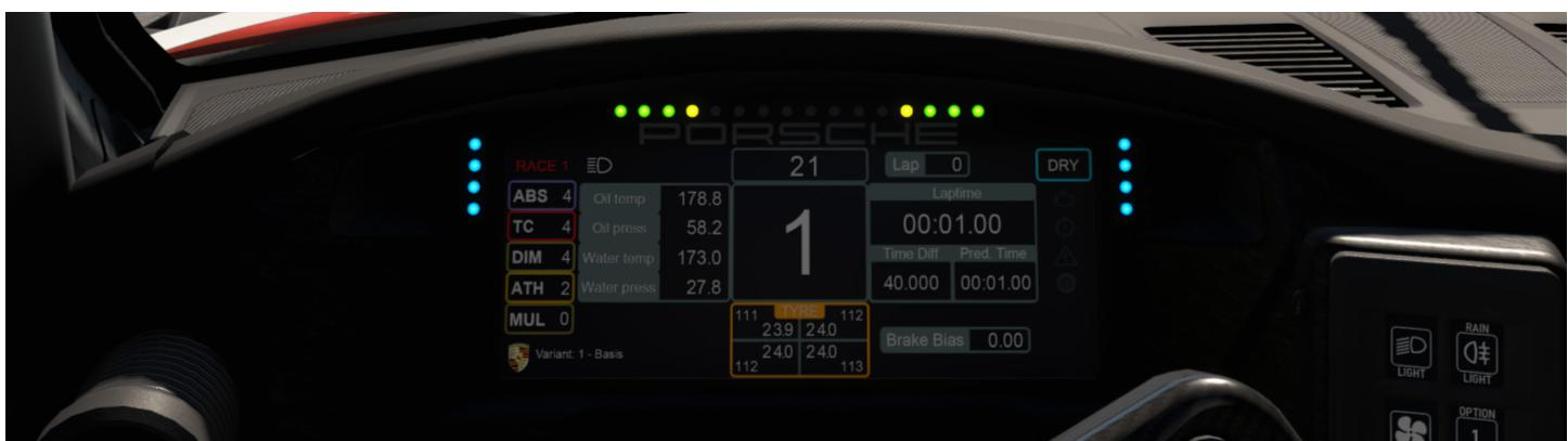
When the traction control system is active, a cluster of blue LEDs on either side of the instrument binnacle. This overrides any wheel lockup lights that may be active at the time.
