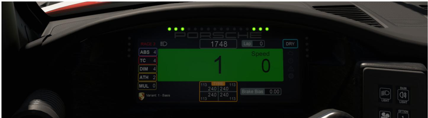
When the pit limiter is active the data displays in the center will be replaced by a large box featuring the selected gear in the center and the vehicle speed on the right. If the speed is at or under the pit road speed limit the box will be green and if the speed is above the
