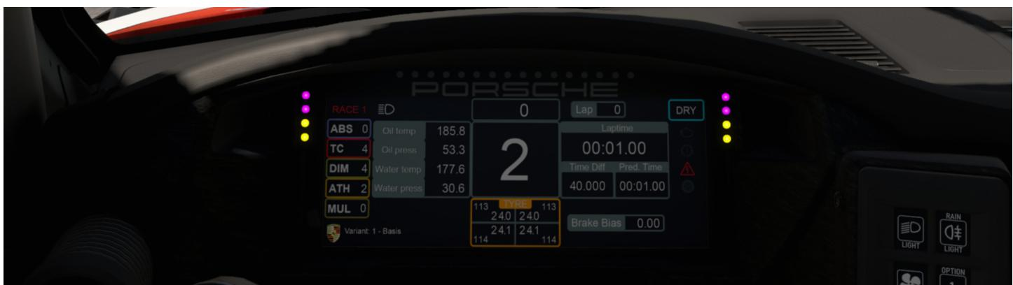
Should one of the wheels begin locking under heavy braking while the ABS system is disabled, status lights on the sides of the display will illuminate to signal which wheel is locking. The front wheels are
