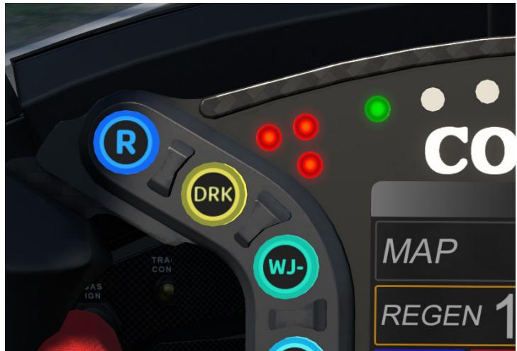
A three-LED cluster on the left side of the display indicates whether the hybrid system is in Deploy or Regeneration mode. During Regeneration (either deceleration or manually-activated regen) the lights will illuminate in Red. During Deploy, the lights will illuminate in Green.
