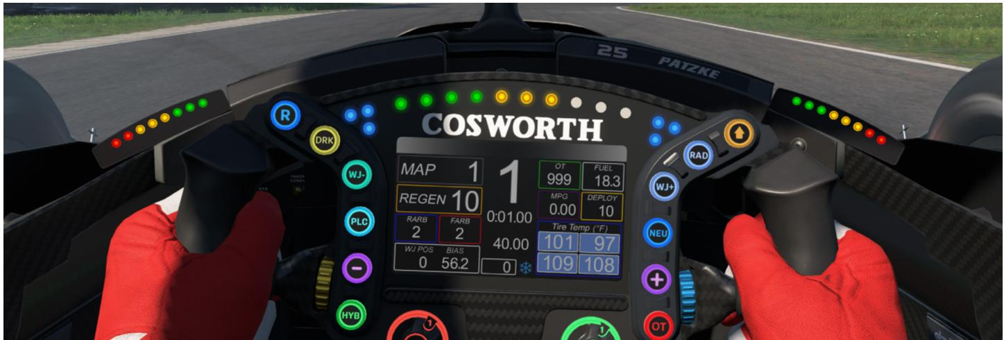
Two LED clusters on either side of the cockpit display the current State of Charge in the hybrid Supercapacitor. When the system is not deploying, the LEDs will be colored red, yellow, and green to indicate the state of charge. A full charge is all eight LEDs illuminated with lights extinguishing as charge is depleted. The lights will keep this color scheme during energy regeneration.
