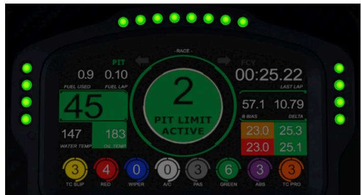
When the vehicle is traveling at the pit road speed limit, the screen and side LEDs will be green.
