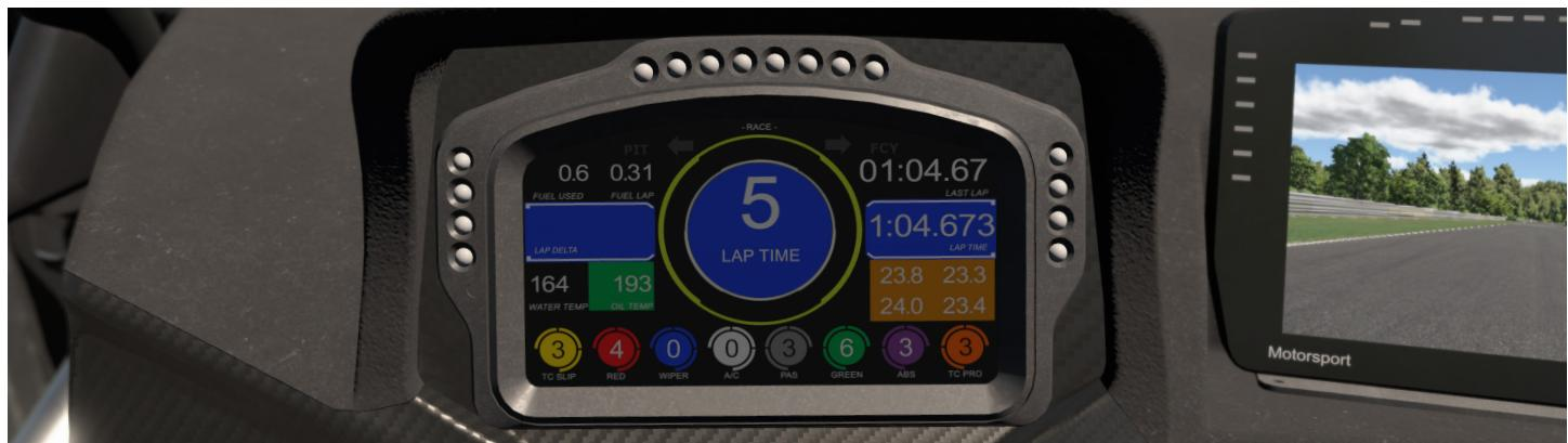
After the completion of a lap, the display will fill three sections with purple and "freeze" to display the previously completed lap time to the driver on the right of the display. This clears after several seconds.
