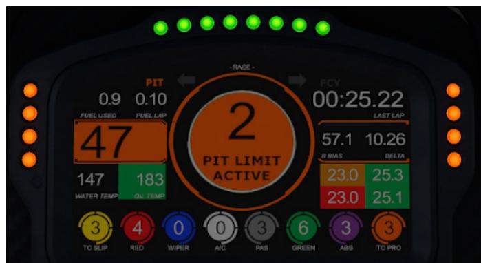
If the vehicle's speed is higher than the pit road speed limit, the display will change to orange with the side LEDs flashing orange.
