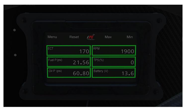
ECT - Engine coolant temperature in °C or °F
