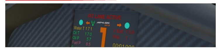
When the pit limiter is active a message in red will appear at the top of the dashboard screen along with two cyan dots and two orange arrows.
