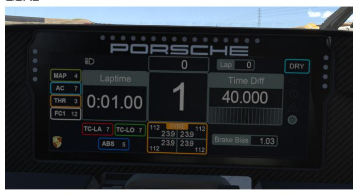
The Qualifying page contains most of the information seen in the Race pages but replaces the Engine and Fuel information with Lap Time, and the Race page Lap Time cluster is replaced with a live split.
