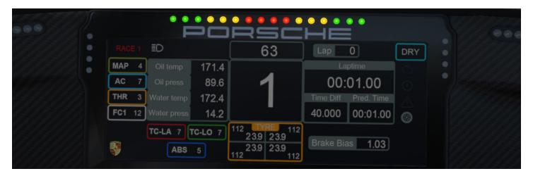
As RPM increases the LEDs will light up from the outside to the inside (green to red), converging just prior to the ideal shift point.
