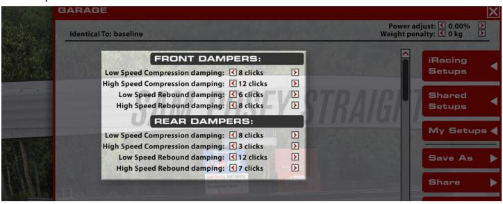
The 4-way KW dampers homologated for this car have 18 possible settings for each adjustment. Setting "O" provides maximum damping and setting "18" is the minimum damping for each adjustment.
