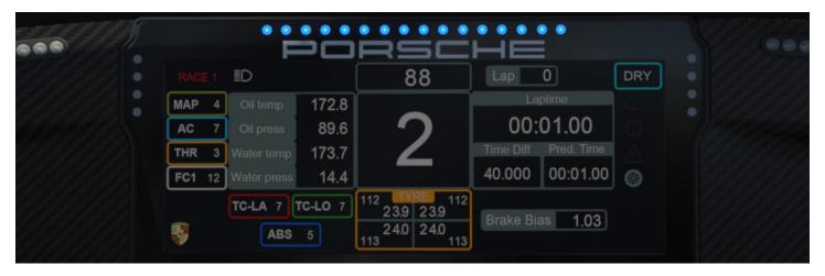
When the ideal shift point has been reached, all shift light LEDs will change to blue and begin flashing.
