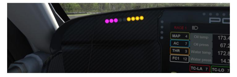
Whenever either the front or rear wheels lock under braking the side clusters will split and show pink for a front axle lockup and yellow for a rear axle lockup. These LEDs also show the severity by how many LEDs are illuminated: One LED shows relatively small or initial locking while all four LEDs indicates severe or complete axle lockup.
