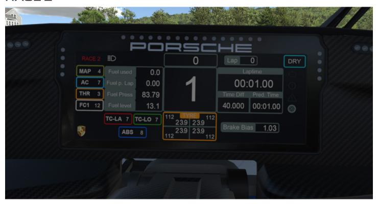
Race 2 is essentially the same page as Race 1, however the Engine Temp/Pressure cluster is swapped for a Fuel information cluster on the left side of the display.
