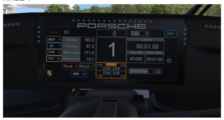
The Porsche 911 GT3 R (992) features an integrated digital dash display with three page options. Two Race pages display information about how the car is running, while a Qualifying page displays information to help the driver know how fast (or slow) the current lap is.
