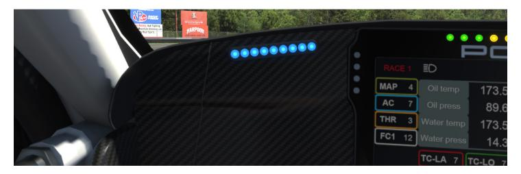
Whenever the Traction Control system is active and attempting to control wheelspin the side clusters will be illuminated in blue.
