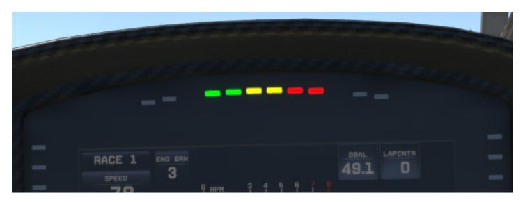
As RPM increases the lights will illuminate from left to right, with all lights turning red when the ideal shift point has been reached.
