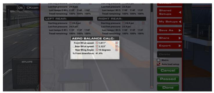
The Aero Calculator is a tool provided to aid in understanding the shift in aerodynamic balance associated with adjustment of the rear wing setting and front and rear ride heights. It is important to note that the values for front and rear ride height displayed here DO NOT result in any mechanical changes to the car itself, however, changes to the rear wing angle here WILL be applied to the car. This calculator is a reference tool ONLY.
