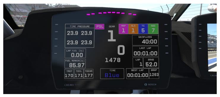
When the pit limiter is active the shift light cluster will flash all LED's in magenta and the PSL box will appear on the main dashboard screen.
