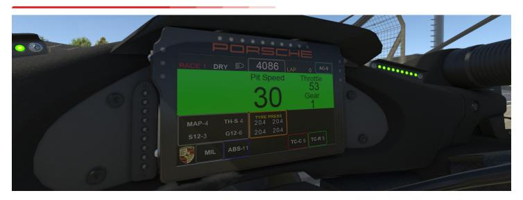
When the pit limiter is active (and you are under the pit speed limit) a large green box that includes the current road speed will display across the top of the dashboard while the left and right lockup light clusters will also illuminate completely in green. Should you be above the pit speed limit the green box will switch to orange.
