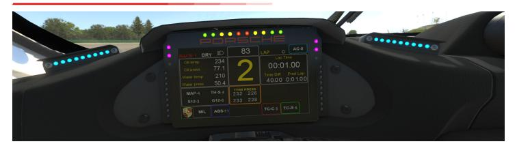
When traction control is active all lights in the lockup light clusters illuminate in blue along with four lights on the digital display illuminating in purple.
