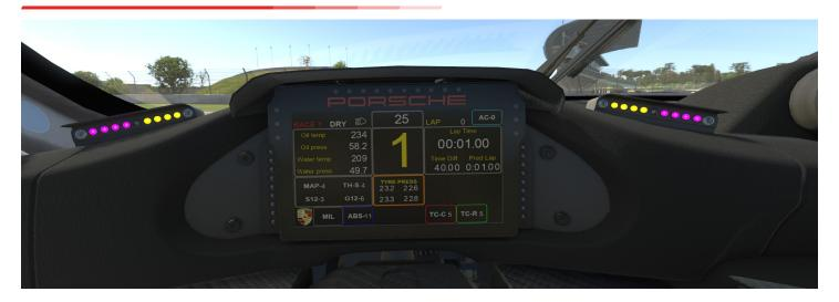
When the front wheels lock, purple LED's illuminate on two pods located on the instrument binnacle corresponding to the road wheel that's locking (e.g. left side lights in purple indicate a front left lockup). The number of lights indicates the severity of the lockup, with one light being a minor lockup and four being severe. This light illumination behaviour is identical for the rear wheels with the exception that these are indicated by yellow LED illumination instead of purple.
