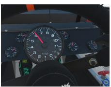
Each Truck features a large tachometer in the center with five accessory gauges arranged across the dashboard. These five gauges consist of:
