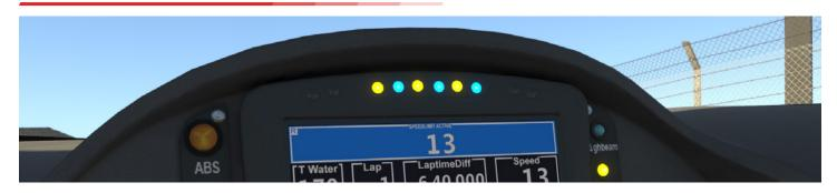
When the pit limiter is active a large blue box that includes the current road speed will display across the top of the dashboard while the center six shift light LED's will illuminate in a yellow and blue sequence.
