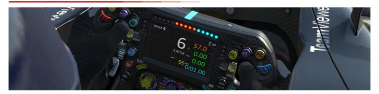
**DEPLOY** - This value represents how many hybrid system deploy mode changes are remaining during the current lap.
