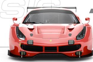
4633mm 182.4in **2045mm** 80.5in 2713mm 106.8in 1283kg 2829lbs WET WEIGHT WITH DRIVER 1406kg 3100lbs
