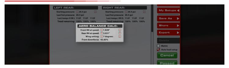
The Aero Calculator is a tool provided to aid in understanding the shift in aerodynamic balance associated with adjustment of the rear wing setting and front and rear ride heights. It is important to note that the values for front and rear ride height displayed here DO NOT result in any mechanical changes to the car itself, however, changes to the rear wing angle here WILL be applied to the car. This calculator is a reference tool ONLY.
