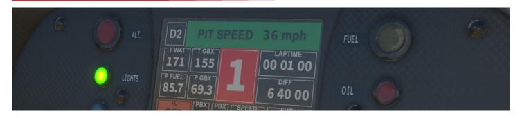
When the pit limiter is active a large green box that includes the current road speed will display across the top of the dashboard while the left and right indicator lights will also illuminate.
