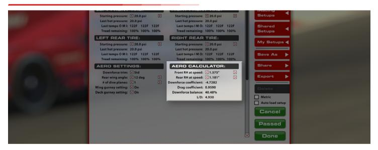
The Aero Calculator is a tool used to display the car's approximate aerodynamic values in a given configuration. Changes to the car's aerodynamic settings (Wing Angles, Dive Planes, Gurney Flaps) will be reflected in the Aero Calculator, giving an idea of how the car will behave aerodynamically while on the race track. This calculator can also be used to determine what changes need to be made to the car to alleviate aerodynamically-induced handling issues.
