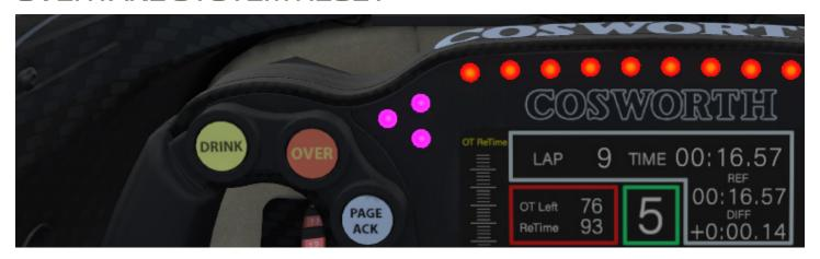
After the Overtake system has been deactivated (but while there is still time remaining for the system to be used) the LED cluster will be illuminated in purple and flash until the system has reset and Overtake can be used again.
