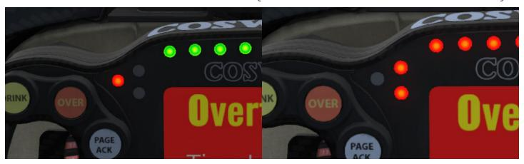
If the Overtake system has less than 20 seconds remaining before deactivation the LEDs will flash in the same pattern as normal operation but will show in red.
