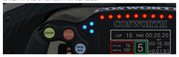
Following the ReTime reset period after the Overtake system is deactivated the LEDs will display in blue to signal the system is available to be used again.
