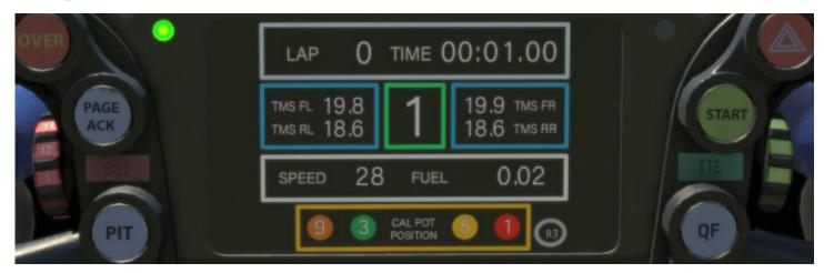
The TMS page features Tire Pressure information in the center row of the display, replacing the Lap Time values on the right side of the dash with right-side tire pressure information. Each value (TMS FL, TMS FR, etc.) shows the current tire pressure in psi or Bar.
