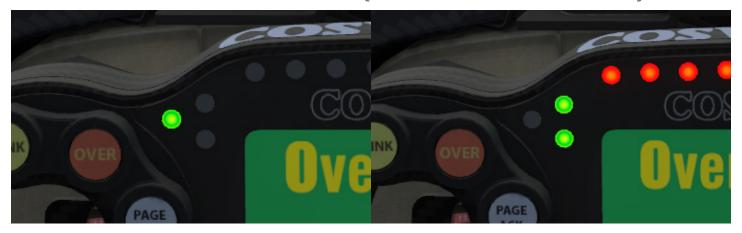
When the Overtake system is activated and the time remaining is over 20 seconds the cluster will alternate left and right in green.
