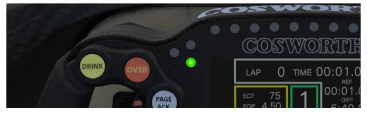
A single green LED on the bottom indicates the brakes are far below optimum temperature and may be inconsistent or not as effective as may be expected.
