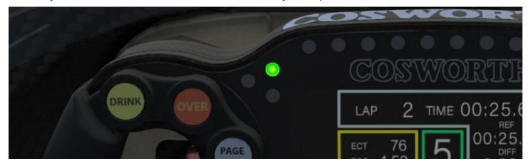
A single green LED on the top indicates the brakes are close to their operating temperature but are slightly cooler than what would produce peak performance.
