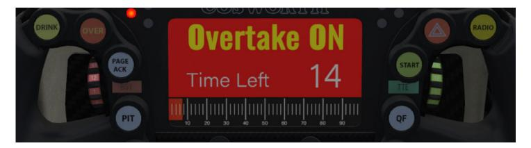
Once the system is depleted, the display will return to the active display page and engine power will return to its standard output. The "OT Left" and "ReTime" values on the Overtake display page will both display "O" for the remainder of the session.
