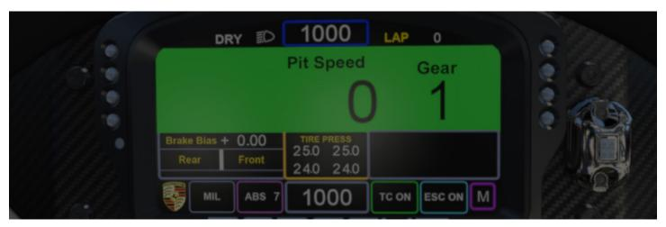
When the pit limiter is active a large green box containing the current speed and gear will fill the upper portion of the dashboard. The box will turn orange if traveling above the pit road speed limit with the limiter active.
