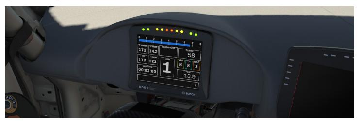
The shift lights illuminate from the outer edges towards the center in the following pattern:
