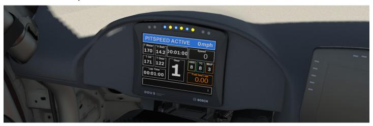
When the pit limiter is active a blue bar will appear at the top of the screen specifying the current vehicle speed. This bar will be blue while under the limit and red when over. In addition to this, the shift light cluster will flash with alternating blue and yellow lights.
