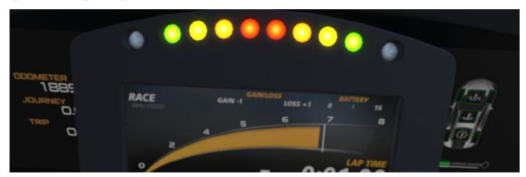
The shift lights illuminate from the outer edges inwardly. Illumination of the first LED will shift depending on the selected gear as such, the below values are only valid for 3rd gear.
