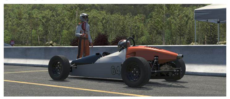
Before jumping into the car, you are encouraged to map a H-pattern shifter and a manual foot clutch (if available). The Formula Vee uses a traditional direct selection transmission with four forward gears plus reverse.
