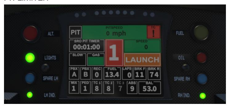
When the pit limiter is active the dash page switches automatically to the 'pitlane' page. This page is only accessible while the limiter is active.
