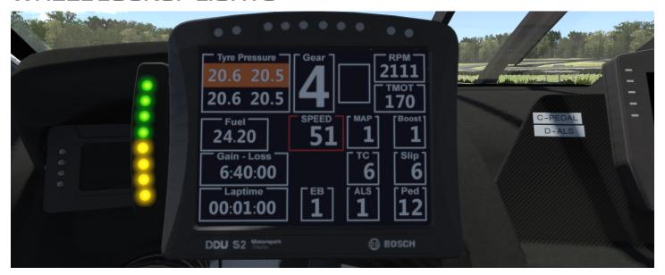
A set of wheel lockup lights are mounted on the left side of the display cluster. These LEDs will illuminate whenever a front or rear lockup is detected, with the lockup's severity being shown by how many lights are illuminated. Initially the top and/or bottom LEDs will illuminate, more severe lockups are shown with more lights toward the middle of the display. The Green lights represent the front wheels and the Yellow lights represent the rear wheels.
