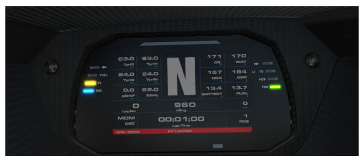
When the pit limiter is active a red banner will appear at the bottom of the display along with illumination of the PSL light on the left side of the dashboard.
