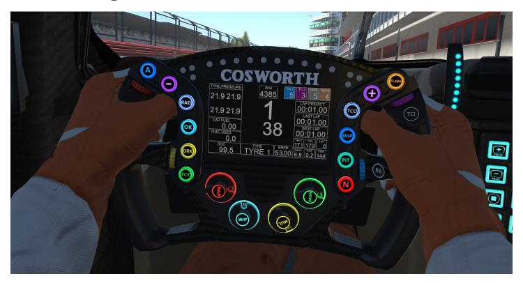
The BMW M Hybrid V8 features a single-page, steering wheel mounted display to provide the driver with useful information in an easy-to-read format.
