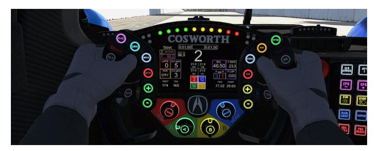
The top of the steering wheel has a set of lights to help the driver know when to shift up to the next gear while accelerating. As RPM increases, the lights will illuminate from the left to right starting with green and ending with two red LEDs on the right. Once the optimum shift point has been reached all LEDs will change to red and begin flashing.
