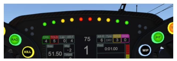
As RPM increases, the LEDs will illuminate from the outside to the inside from green to red. More lights will illuminate as the optimum shift point is approaching.
